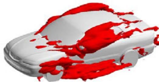
Fig. 4 Iso-surface of Lighthill-Curle's acoustic source (CFD result)
