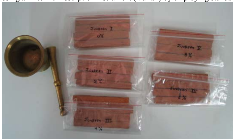
Figure 2. Samples of final ceramic bricks prepared using different percentages of clay and powder activated sludge.
